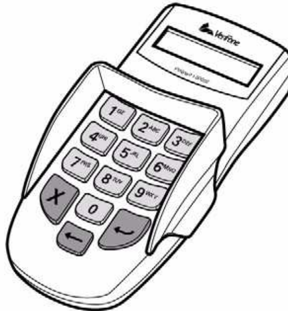
Figure 7 Installed Privacy Shield
